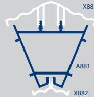
135° FLUTED BAY COUPLER Use with 4310 Jack Assembly and 4311 (2 off) Bearing Plates
